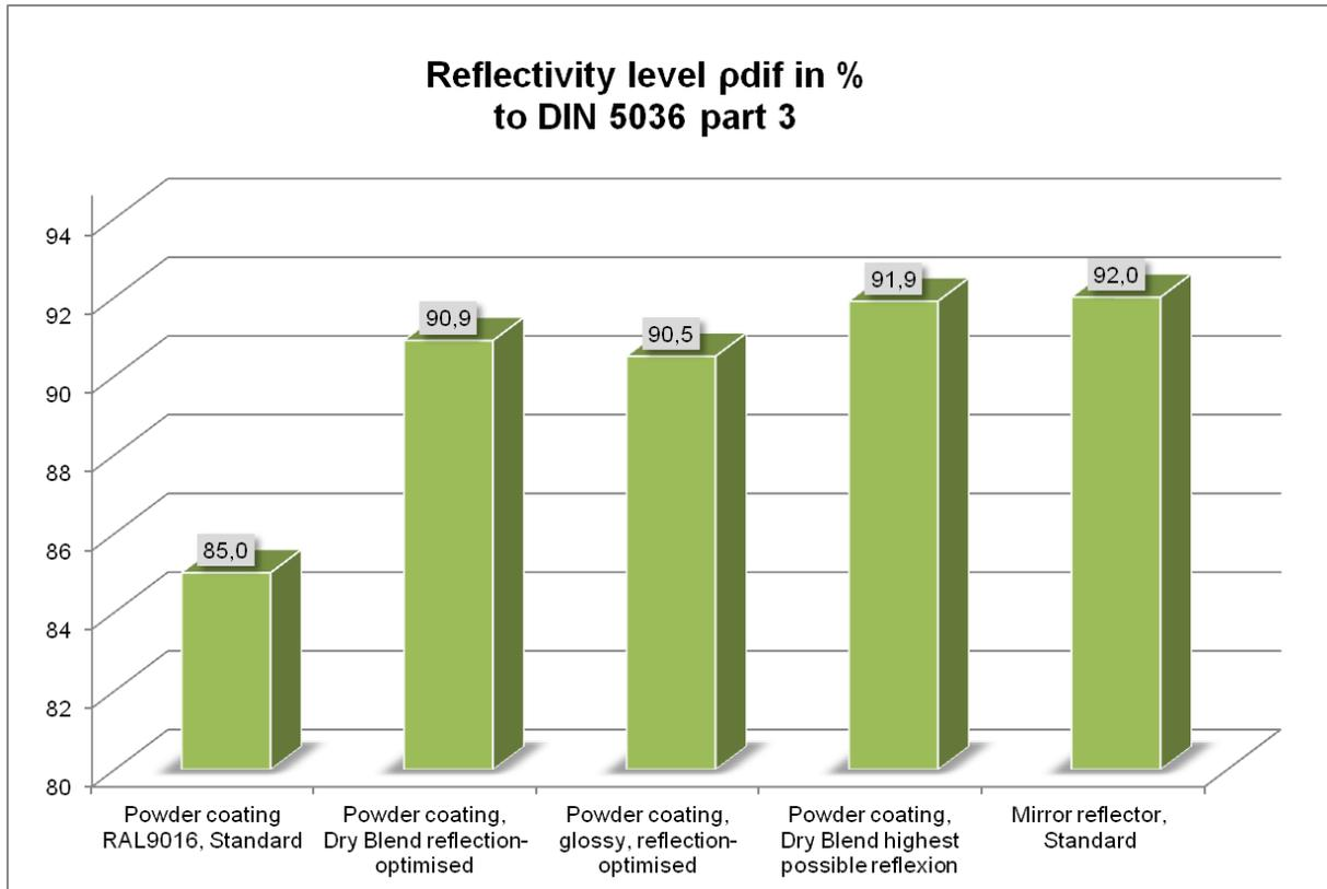
Fig. 4: Different reflectivity levels of powder coatings
