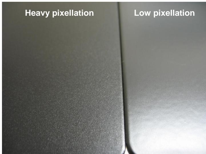
**Fig. 3: Pixellation differences between dry-blend powder coatings**
