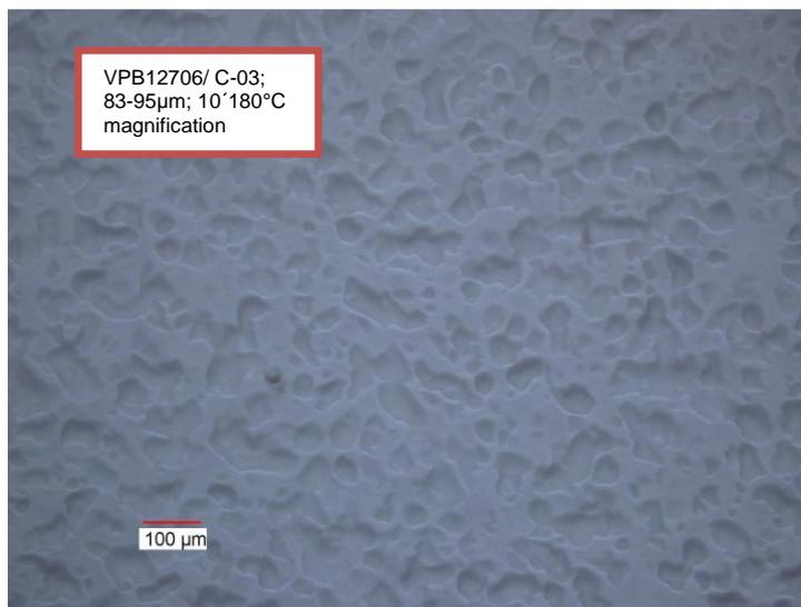
**Fig. 2: Microscopic image of the microstructure of dry-blend powder coatings**
