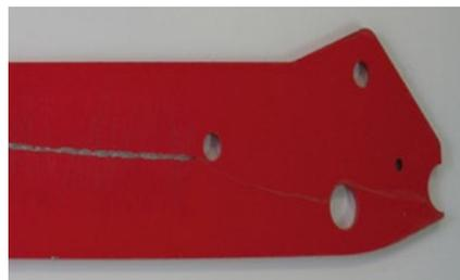
Production component after a 504-hour salt spray test.
