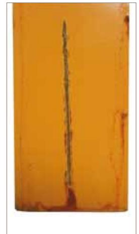
Salt spray test on single-coat system after 500 h
